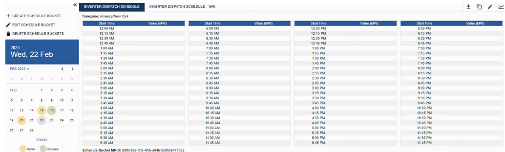
Figure 13. Distributed Energy Resource Management (DERM) Control User Interface (UI), displaying the feature to set the desired dispatch schedule provided by Strata Grid.
