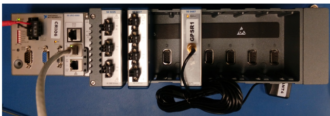
FIGURE 3: Physical PMU hardware in a Compact-RIO 9068
