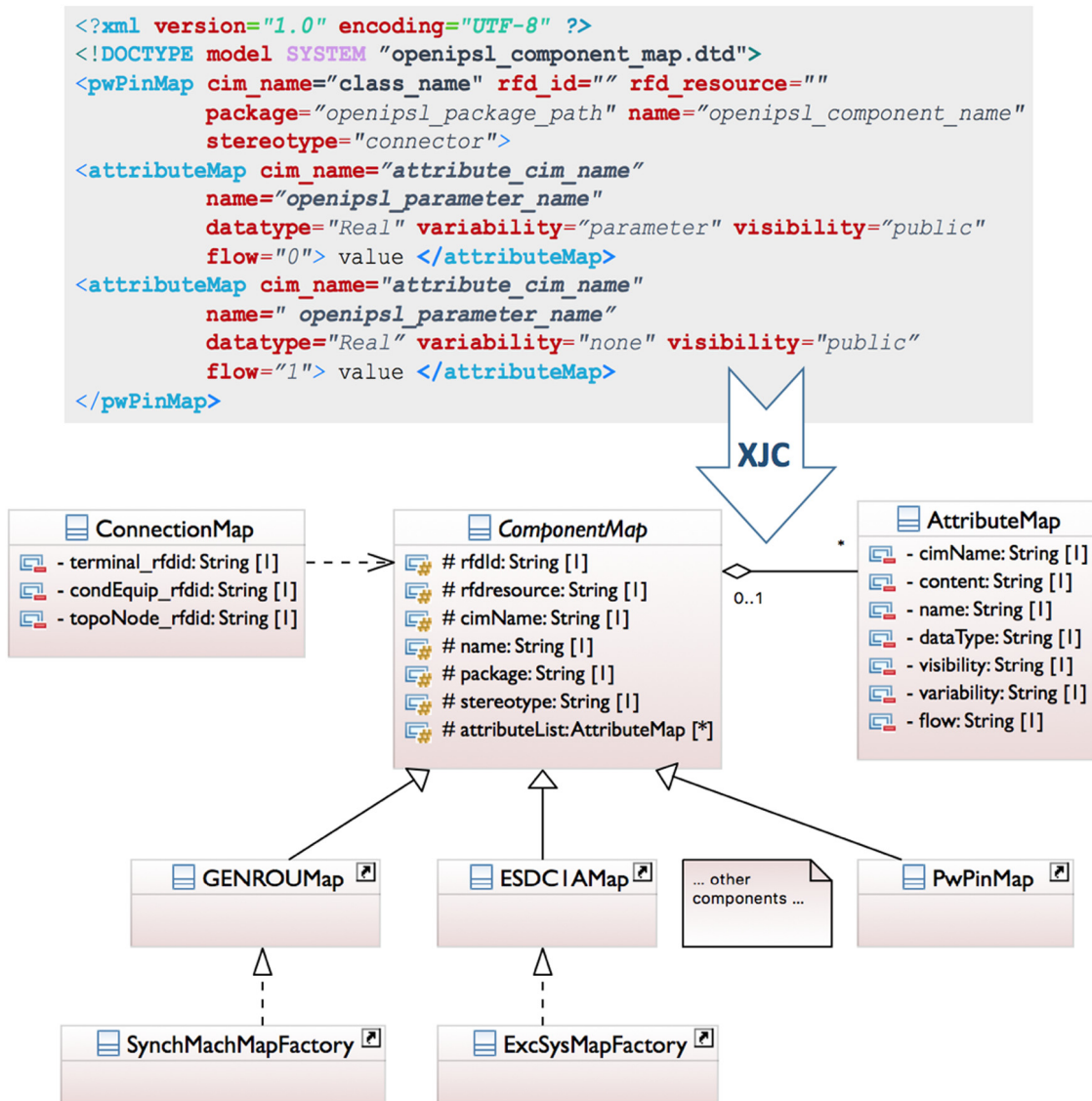
Fig. 3. On the top of the arrow, an example of an XML Mapping rule file with general syntax. On the bottom, the final version of the Mapping Meta-Model class structure resulting from the execution of the XJC command for generating JAVA classes from XML schema.
