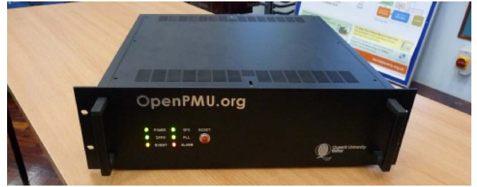
Fig. 2. OpenPMU unit in 19" rack form factor enclosure.
