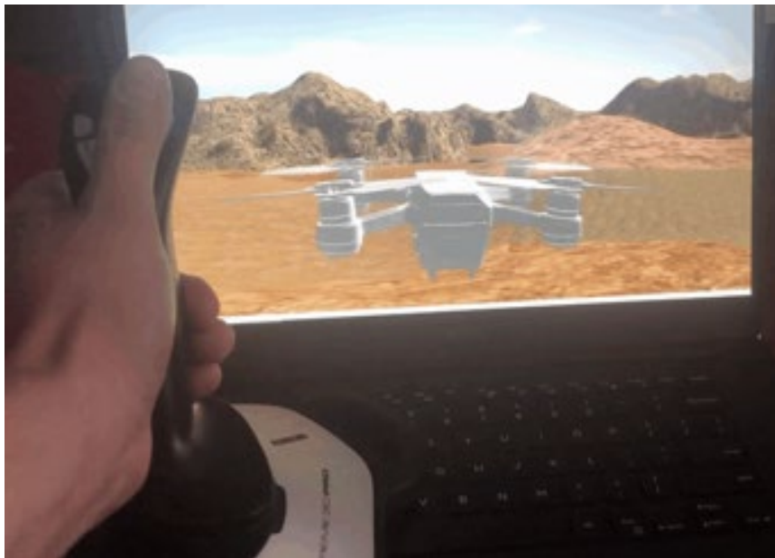
Figure 14: Drone model in simulated terrain environment using the DLR Visualization Library controlled by joystick input
