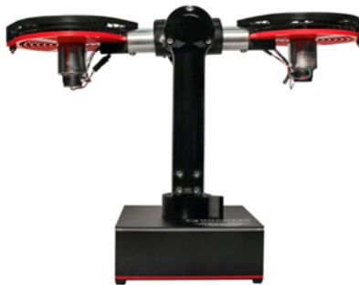
Fig. 1 The Quanser AERO in a 1-degree-of-freedom configuration.
