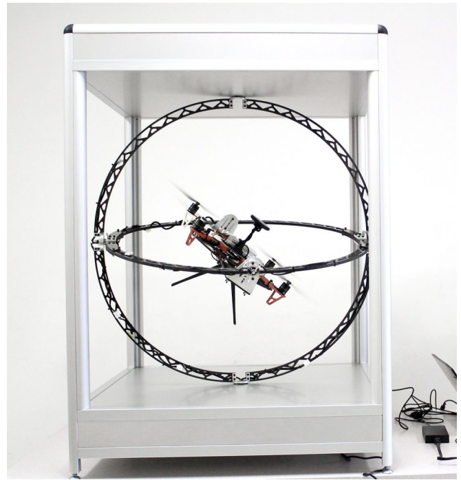
Figure 3. FFT gyroscope test bed setup (Ref. 11).
