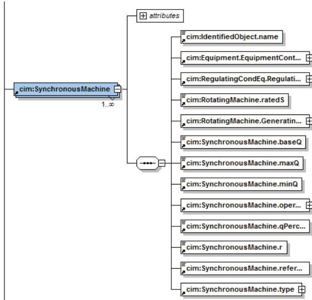
Fig. 2. Graph structure of the attributes of the CIM class SynchronousMachine.
