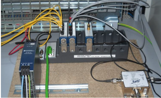
Fig. 1. cRIO 9074 PMU connected to the emulator.
