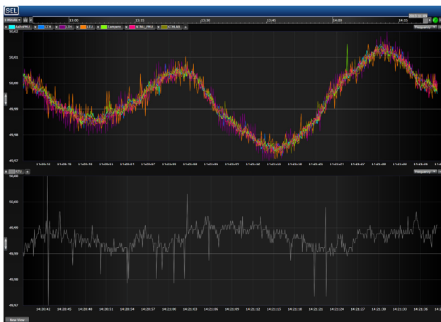
Fig.3: Graphical visualization of synchrophasor data available through university PMU network. The upper half shows the frequency measurements received from the PMUs at KTH (Stockholm, Sweden), LTH (Lund, Sweden), LTU (Luleå, Sweden), Tampere (Finland), AALTO (Helsinki, Finland) and NTNU (Trondheim, Norway). The lower half shows the frequency measurements from the PMU at Riga Technical University (Riga, Latvia), which is not the part of same synchronous power system as Sweden.
