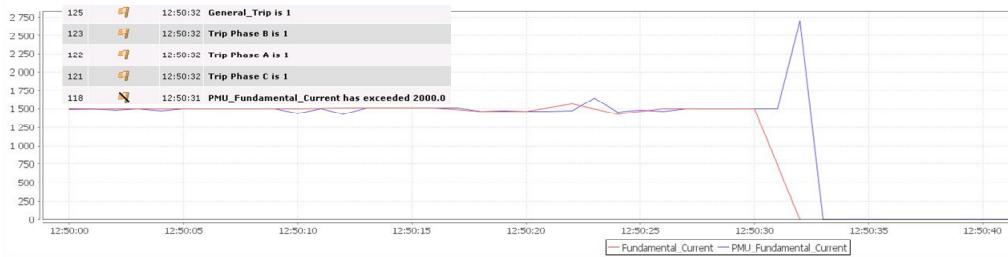
Fig.9: SCADA monitoring of fundamental current measurement received from DNP3 and PMU (IEEE C37.118) protocols
