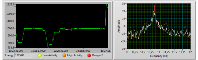
Fig. 9. Partial screen shot of the Monitoring Tool during the oscillation injection at 10.83 Hz and minor faults
