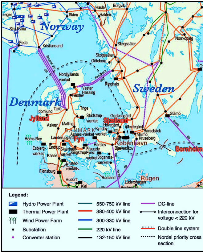
Figure 1. The Danish power grid and its interconnections
