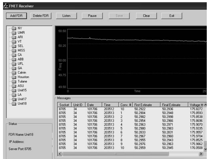
Figure 2. FDR small server program retrieving data at ATBU
