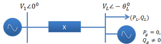
Figure 2.4 Connection of a fictitious generator to calculate the QV curves
