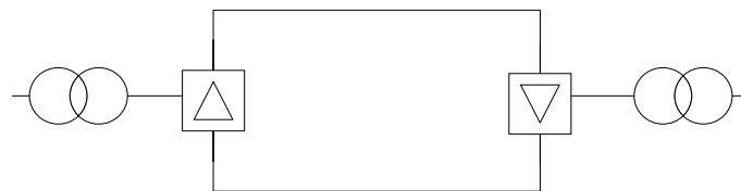
Figure 2.3: Back to back VSC-HVDC system.
