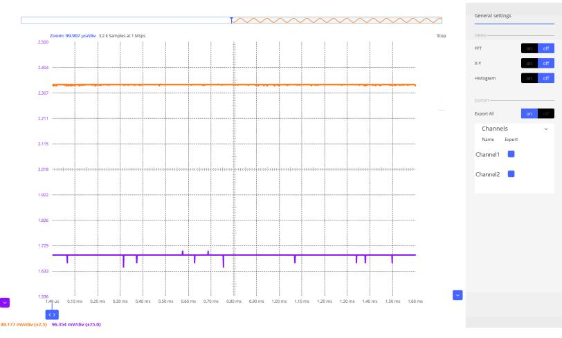
Above is a screen shot of the oscilloscope output from Scopy where the orange graph represents the voltage across R1 and the purple line represents the voltage across R2. Using the tab shown on the right I was able to export the data as a text file. Text files are compatible with Matlab and can be graphed when importanted and converted to column vectors, which can then be graphed with a simple program. The code used in Matlab and the output graph are shown below.
