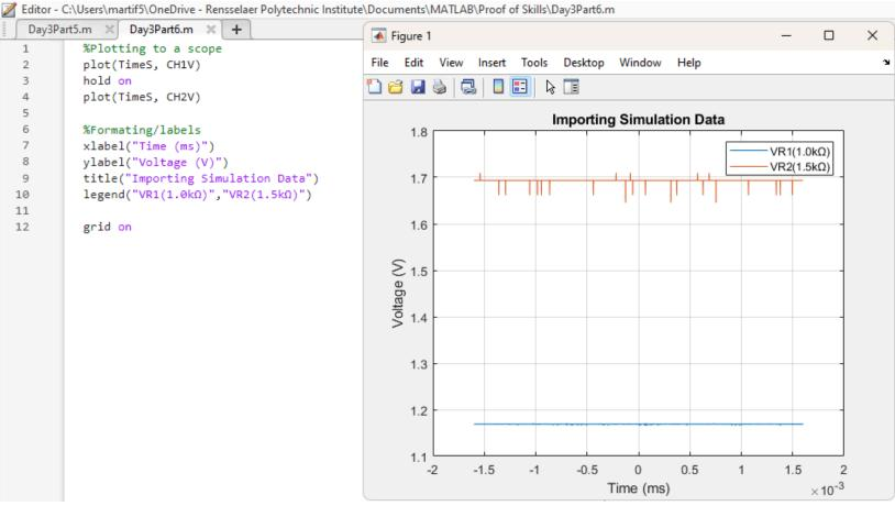
As the above graph shows, the Matlab plot is identical to the plot provided by Scopy.
