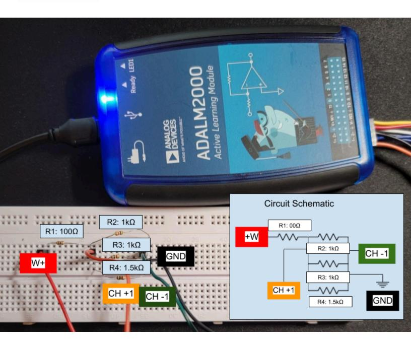
Below we see that all sources of measuring the voltage across R2 are within reasonable tolerances of each other, where the LTSpice simulation is the accurate and real-world test shown to lose some voltage from wire resistance and other non-conservative materials.
