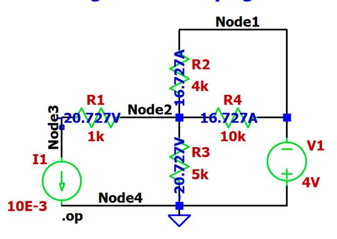
Above is a circuit simulation that contains many components such as resistors, batteries, and current source. Each node is identified with black text using the naming convention Node#. A node can be identified at a point in between two or more circuit components.
