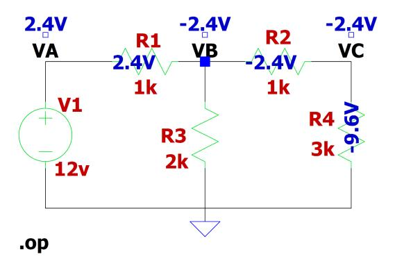
I was able to identify nodal voltages, VA, VB, and VC, with the blue labels in the image and round them to the nearest decimal place by going in to the Display Data setting and typing round(V(#)\*10)/10 into the edit expression box. I also was able to label the voltage and resistors which I kept R and its number as well as the voltage labeled as V1.
