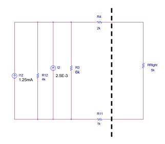
Step 4: After combining current sources and resistors, convert to voltage source so R4 and R11 can be added
