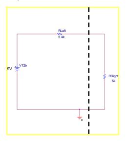
If you used P-Spice to check your answer Voltage divide solution to A and it should be the same as the voltage of the node right above R5 in original diagram. 4.327V
