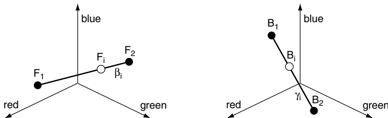
Figure 2.12. The color line assumption says that each pixel I_i in a small window of the image is a mix of a foreground color F_i and a background color B_i , where each of these colors lies on a straight line in RGB space.
