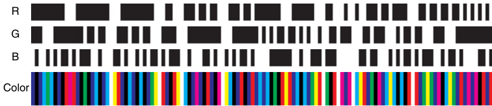
Figure 8.21. Zhang et al.'s color stripe pattern created using a de Bruijn sequence of order 3 over five symbols.
