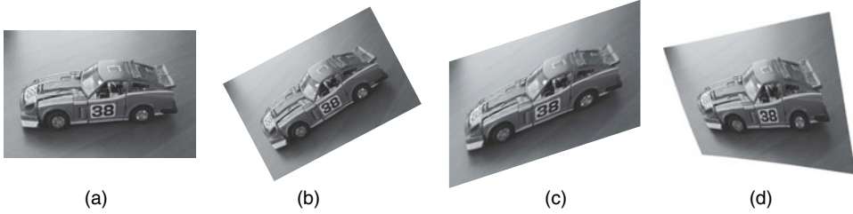
Figure 5.1. An original image (a) and the results of various affine and projective transformations. (b) A similarity transformation (i.e., translation, rotation, and uniform scale). (c) A vertical shear. (d) A general projective transformation. While (b) and (c) can be written as affine transformations, (d) cannot.
