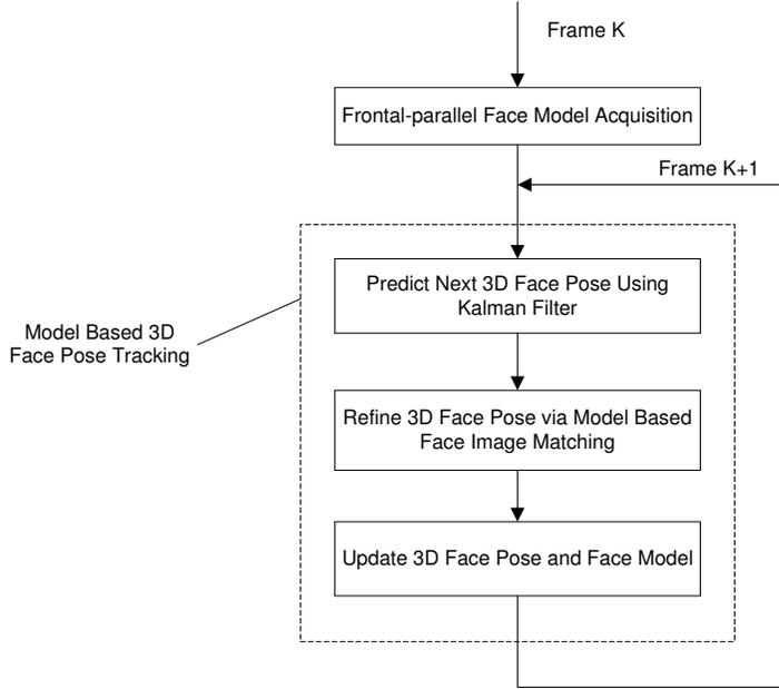
Fig. 10. The flowchart of face pose tracking
