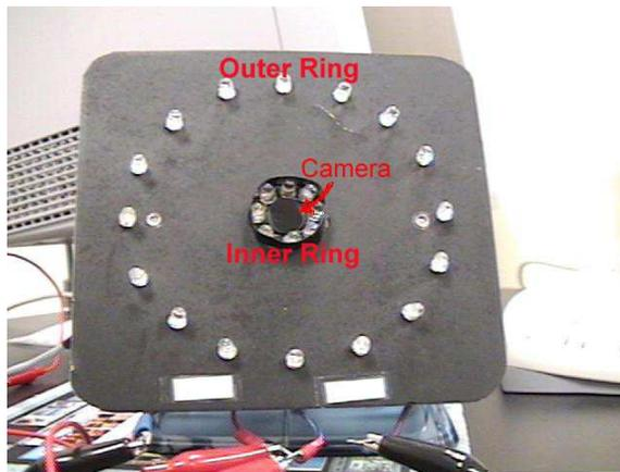
Fig. 4. An actual photo of the two rings IR illuminator configuration
