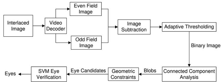
Fig. 6. Eye detection block diagram
