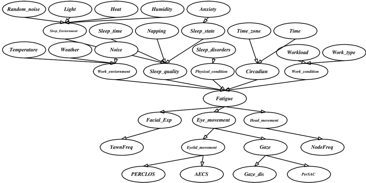
Fig. 22. Bayesian Network model for monitoring human fatigue
