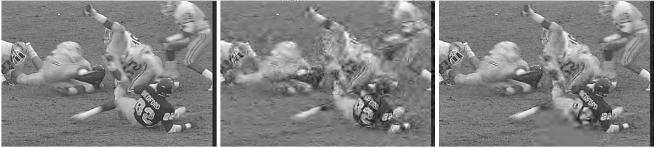
Figure 12. 352 x 240 original “Football” sequence (frame15) (left) 352 x 240 “Football” reconstruction using normal 3-D SPIHT/FEC with BER = 0.01. PSNR = 24.41dB (middle), 352 x 240 “Football” reconstruction (frame15) using STTP SPIHT( n=16 )/RCPC with BER = 0.01. PSNR = 29.35dB (right). Total transmission rate is set to 2.53 Mbps.
