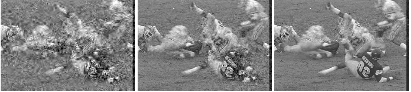
Figure 10. 352 x 240 “Football” sequence (frame15) coded to 1.0 bit/pixel with BER = 0.00001. Normal 3-D SPIHT, PSNR = 18.25 dB (left), STTP-SPIHT ( n = 4 ), PSNR = 23.67 dB (middle), STTP-SPIHT ( n = 16 ), PSNR = 27.00 dB (right)
