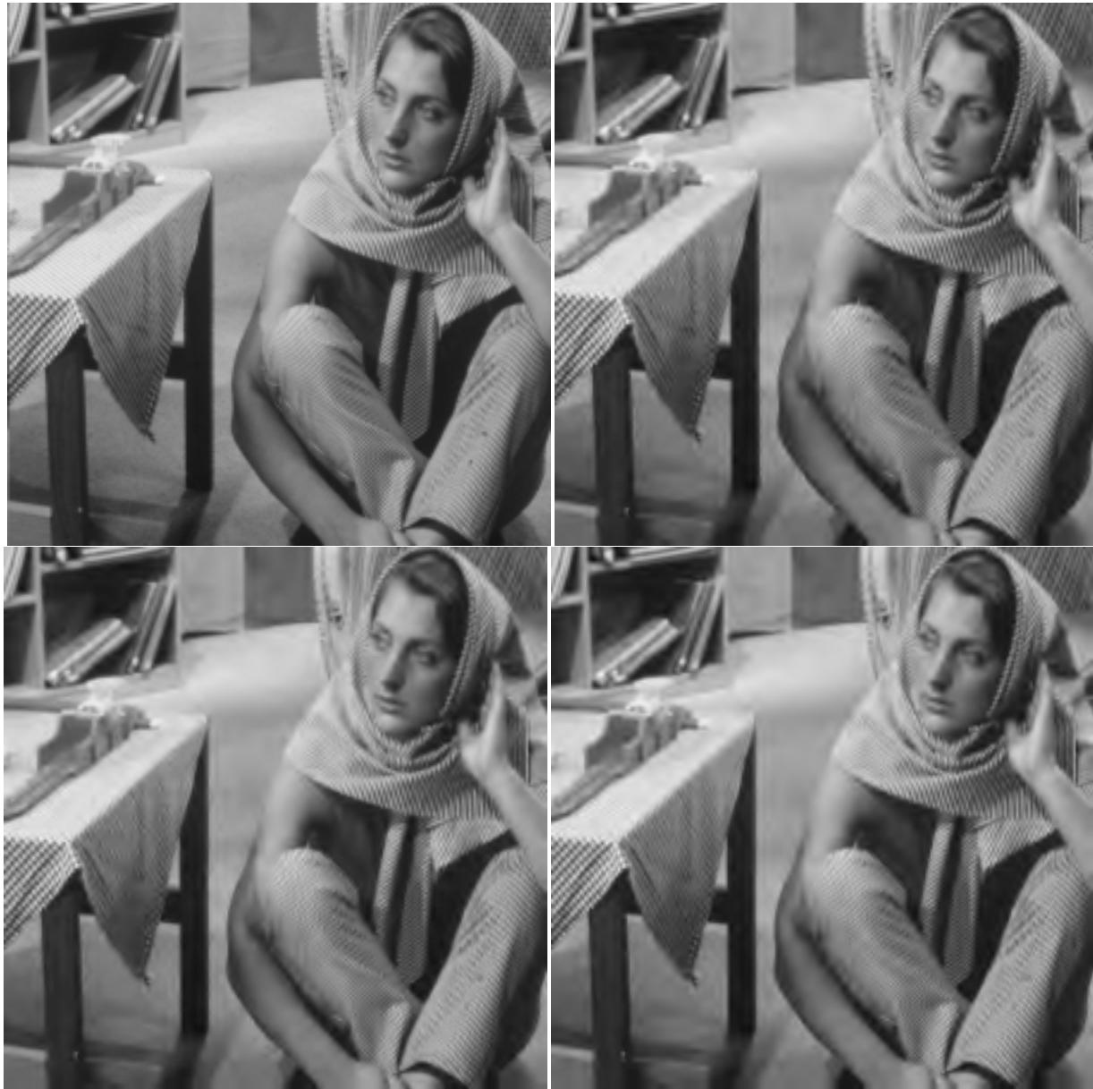
Fig. 7. Comparative coding results of Barbara image at 0.25 bpp: Original (top left), SPECK (top right), SPIHT (bottom left), and JPEG2000 (bottom right).
