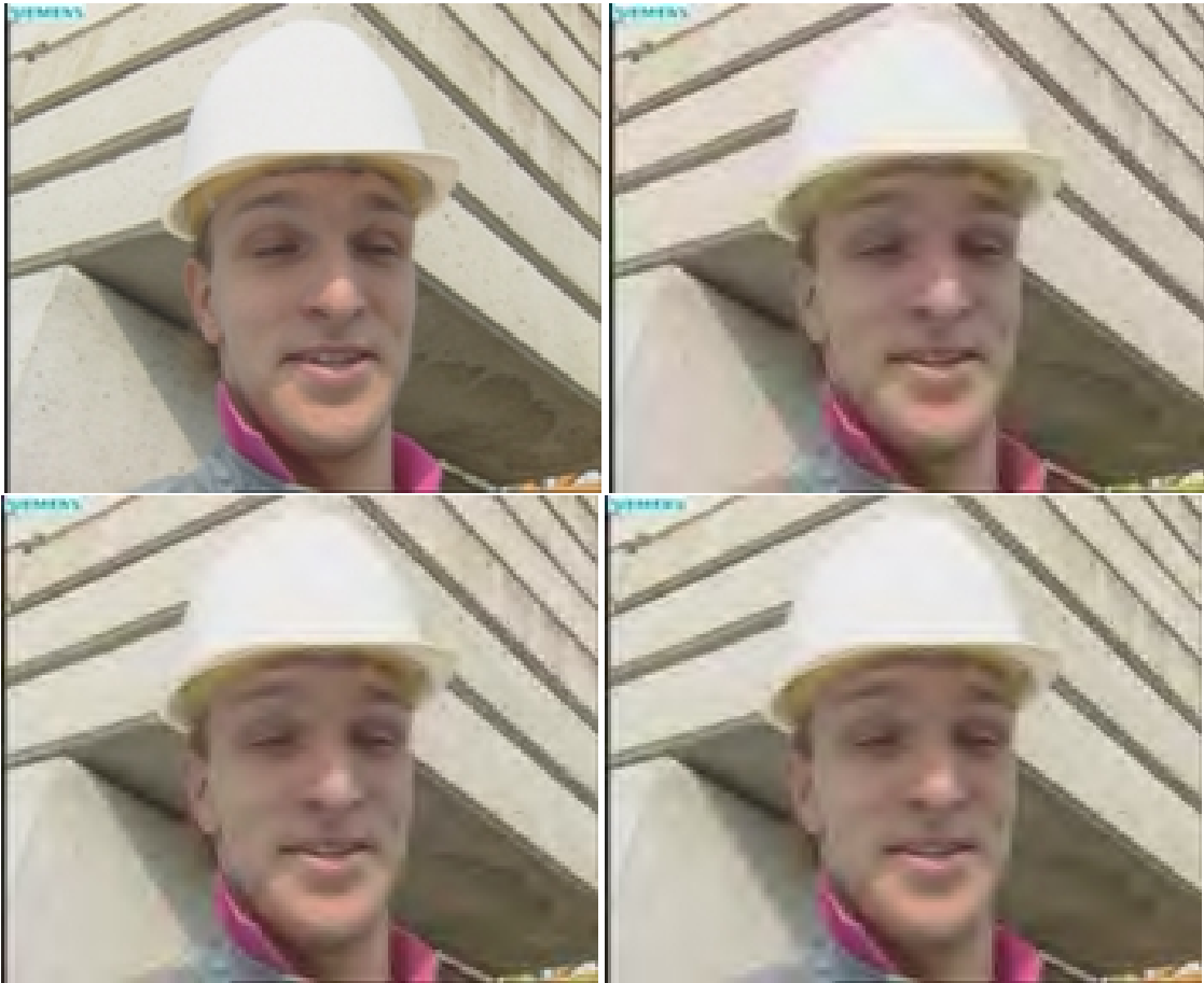
Fig. 11. Reconstructions of first frame of Foreman sequence compressed to 19,300: Original (top left), CSPECK (top right), SPIHT (bottom left), and JPEG2000 (bottom right).
