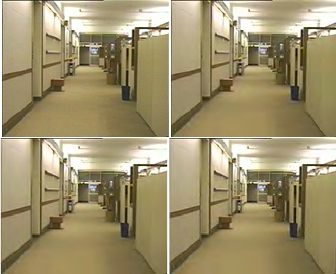
Fig. 12. Reconstructions of first frame of Hall Monitor sequence compressed to 28,500 bits: Original (top left), CSPECK (top right), SPIHT (bottom left), and JPEG2000 (bottom right).
