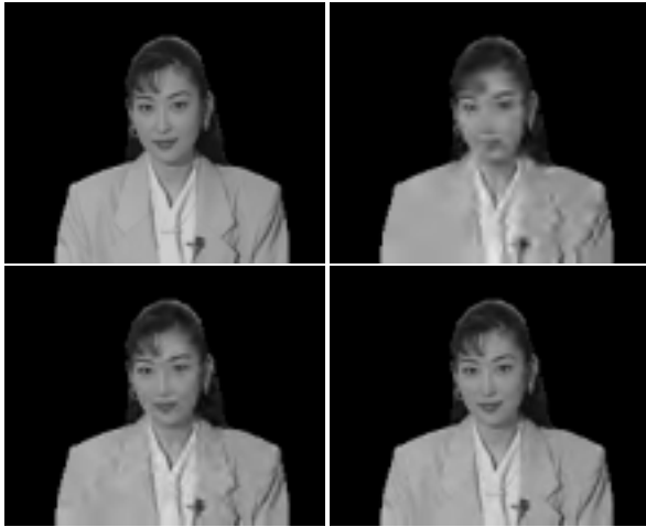
Fig. 3. Original and decoded frame 0 of the Akiyo sequence (QCIF): original (top left), 0.2 bpp (top right), 0.5 bpp (bottom left) and 1.0 bpp (bottom right)
