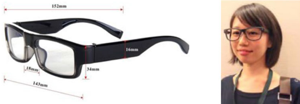
Figure 3. Left: KJR DVR290, 1280 × 720 pixels, 312 g. Right: J!NS MEME prototype, smart glasses.
