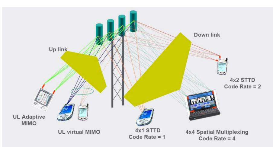
MIMO solutions for both DL and UL to deal with diverse BTS and device antenna capabilities and enable ubiquitous interoperability
