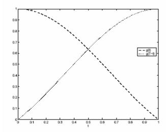
$$\begin{array}{ll} \text{(c)} \ \ g(t) = \frac{\sqrt{\pi}}{\alpha} e^{-\pi^2 t^2/\alpha^2} & 0 \leq t \leq T \\ g(T-t) = = \frac{\sqrt{\pi}}{\alpha} e^{-\pi^2 (T-t)^2/\alpha^2} & 0 \leq t \leq T \\ \text{plotted for T=1 , integral value} = 0.009 \end{array}$$
