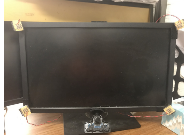
Fig. 2. Hardware setup with one web camera and 4 IR-lights on the 4 corners of the monitor.
