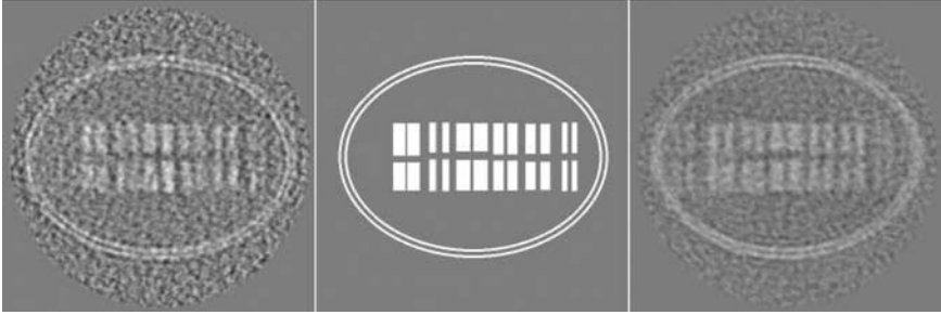
FIGURE 10. One slice perpendicular to the Z-axis corresponding, from left to right, to the ART reconstruction, the phantom volume and the WBP reconstruction, respectively.
