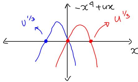
$$\frac{dV}{dt} = -(1-\theta)x^4 - \theta x^4 + xu \leq -(1-\theta)x^4, \quad \forall \|x\| \geq \left(\frac{|u|}{\theta}\right)^{1/3}$$
