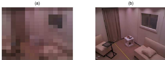
Fig. 3. (a) A sample 15 \times 15 reading of the diffused sensor array. (b) the corresponding image captured.
