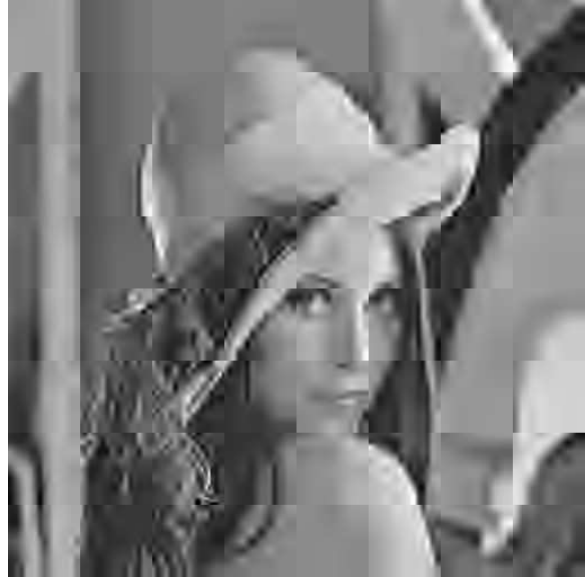
(b) JPEG2000 with a tile size 64 \times 64 pixels. Bit rate is 0.1\text{bpp} . PSNR = 25.12\text{dB} .
