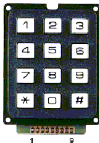
Figure 5.14 - Wiring for keypad. Pins 1 and 9 are unconnected. Only pins 2-8 are used.
