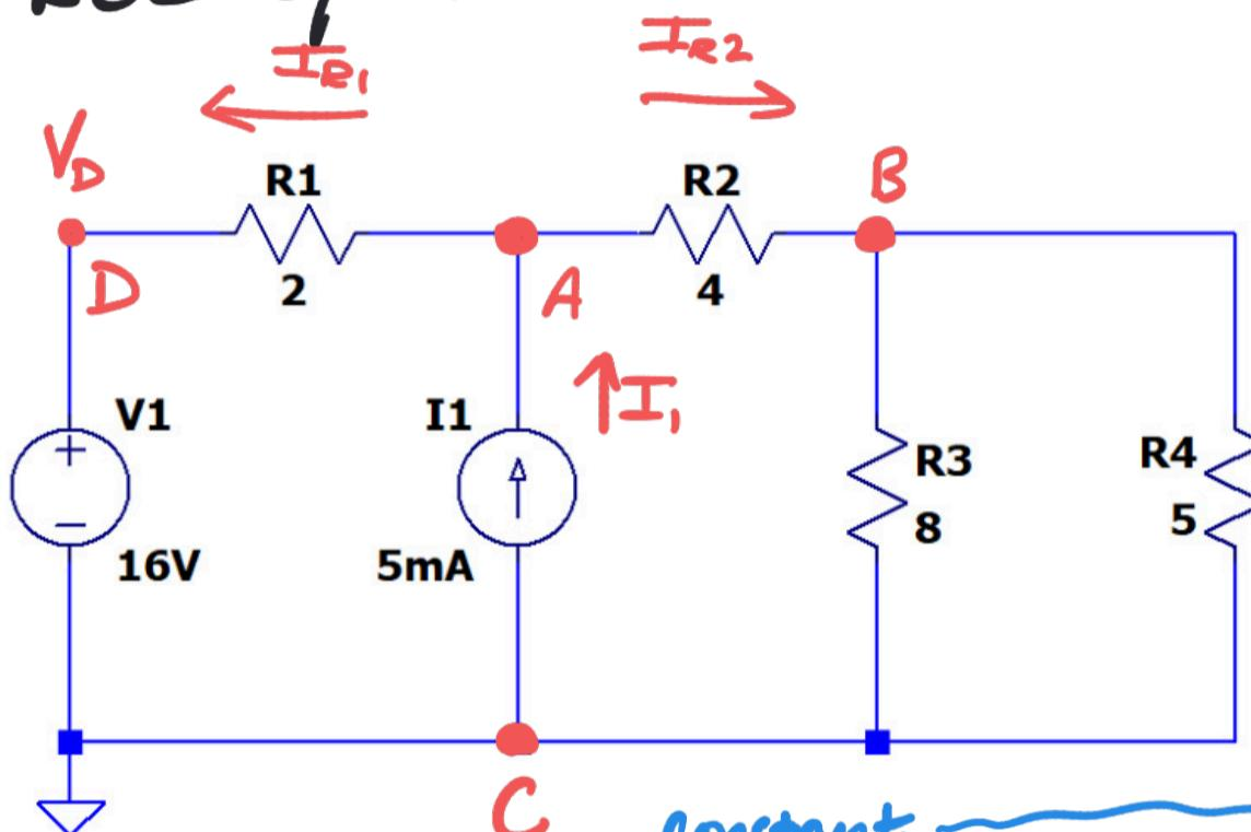
$$\text{KCL @ } A: \frac{V_A - V_D}{R_1} + \frac{V_A - V_B}{R_2} - I_1 = 0$$
