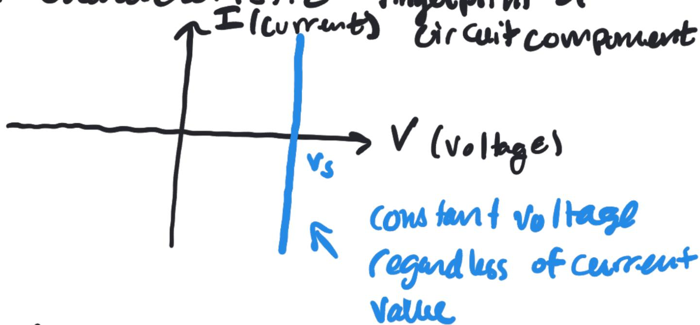
→ Examples: DC power supply, battery, function generator
