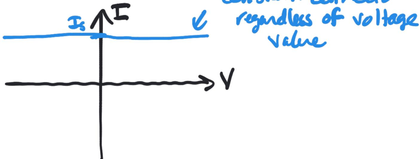
→ Examples: photodiode, transistors
