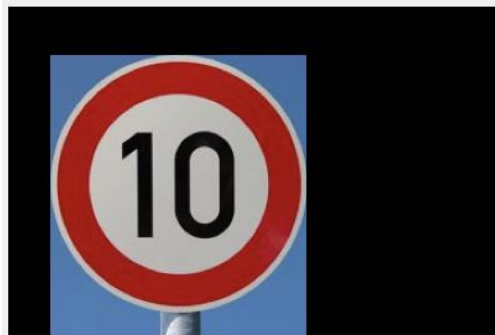
Figure 17: Original RGB image masked by the bounding box of the largest area of connected pixels
