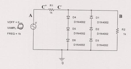
Six 1N4002 diodes are used to protect a load (in this case R2) from having too large a voltage across it. The 4002 diode has somewhat different properties than the 4148 diode we have studied in class.
