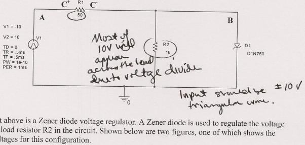
The circuit above is a Zener diode voltage regulator. A Zener diode is used to regulate the voltage across the load resistor R2 in the circuit. Shown below are two figures, one of which shows the correct voltages for this configuration.
