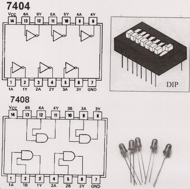
Also used are LEDs to show when voltages are high or low, DIP switches (that fit nicely into protoboards), and wires. The top rail on each board is 5V and the bottom rail is ground.
