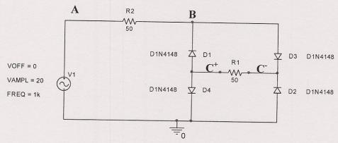
1. A rectifier bridge is used to produce a DC voltage from a sine wave with an amplitude of 20V. The circuit is analyzed with and without a smoothing capacitor.
