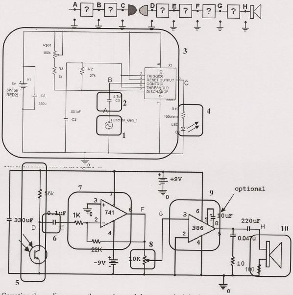
Counting the audio source, the speaker and the two optical devices, there are 10 separate blocks in this communication system.
