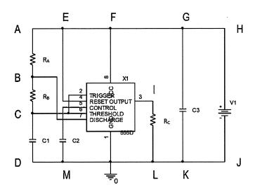
e. Modify the circuit to achieve a 90% duty cycle. You are only allowed to change only one resistor and no other components. The frequency is allowed to change. Which resistor do you change and what is the new value? (4 Pts)
