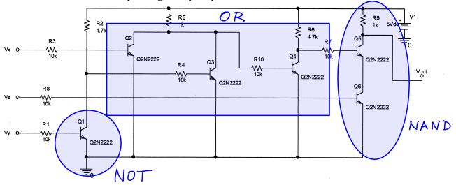
i) (6 points) Draw the logic diagram for the above circuit. Use logic gate symbols and show how the inputs X, Y, Z are related to output OUT. For this you need to identify how transistors, and serial/parallel connections of transistors, can be used to implement logic functions.
