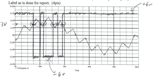
c. This is now the same circuit but configured as a Schmitt Trigger. Vc is the voltage at the non-inverting input of the op amp. Ra=1k $\Omega$ . The goal here is to determine values of Rb that will eliminate false output transitions caused by the noise signal.
