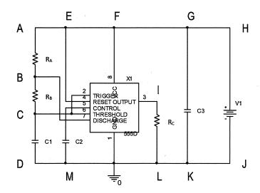
a. A 555 timer, a stable multivibrator is built as above with  $R_A = 10 k\Omega$ ,  $R_B = 9.1 k\Omega$ ,  $R_C = 40 k\Omega$ ,  $C1 = 0.1 \mu F$ ,  $C2 = 0.01 \mu F$ ,  $C3 = 330 \mu F$ , and V1 = 9V. Determine the **on time** (T1) and the **off time** (T2) for this circuit. (4 Pts)
