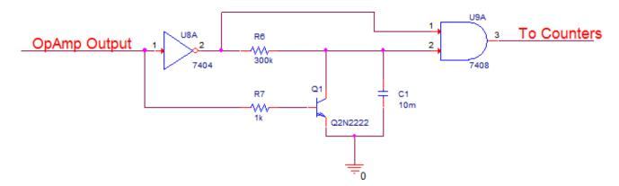
Not: that this circuit should have had another inverter on the opAmp input. Iit was designed assuming that nighttime produced an OpAmp output of HIGH instead of the requested solution shown in pt 1&2. Due to this, LOW represents daylight. Any answer that was obviously confused because of this was accepted.
