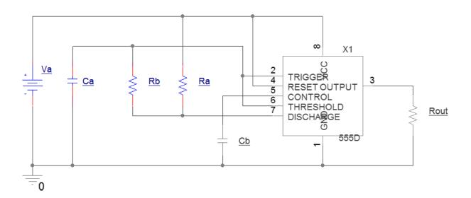
2.2 (4 pnts) Using the labels defined in 2.1, write the equations for the frequency and duty cycle of the output of the circuit above.
