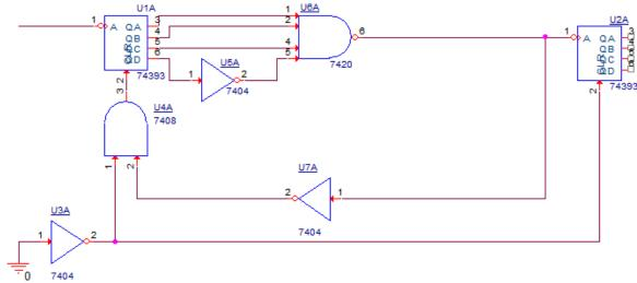
4.6 (2 pnts) The below circuitry was inserted between the op-amp subcircuit and the counter subcircuit. What is it's purpose and how does it work? Hint: the sensor may be placed were it is generally dark at night, but cars may drive by frequently.
