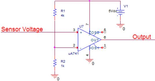
Compare voltage needs to be in the range of 0.75-1.5 V. Using 1 V. Select a reasonable value for R2 and calculate R1. A Schmitt trigger was also be acceptable here. For grading, inverted outputs were also accepted as they were the bulk of the answers.  $R_2$
