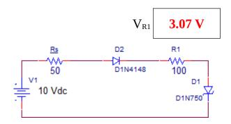
$$V_{R_s} + V_{R_1} = 10V - 0.7V - 0.7V = 8.6V$$
