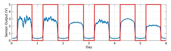
4.1 (4 pnts) The sensor voltage needs to be converted into a digital logic signal before being used to count the days, with logic HIGH voltage representing daytime. Design and sketch an op-amp circuit, with component values, that will achieve this. Select reasonable sized values for the components.
