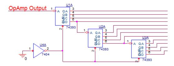
4.4 (2 pnts) The circuit from 4.3 is to be redesigned to count weeks instead of the total number of days. Logic gates need to be inserted between counters U1A and U2A such that the input to U2A is usually a logic HIGH, but transitions to a logic LOW after the last day of the first week counted. What single logic state of U1A's outputs should cause a logic LOW?
