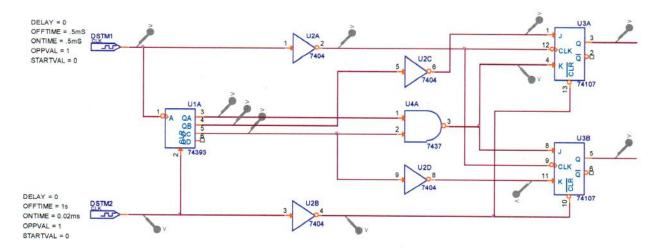
In the circuit pictured above, clock DSTM1 provides a clock signal to a counter and two flip flops. The flip flops are clocked one half cycle after the counter to allow for propagation of the signals through the gates. (The counter changes on the negative edge of DSMT1 and the flop flops change on the negative edge of U2A:Y.) DSTM2 provides an initial reset pulse to both chips. This is required by PSpice to ensure that all sequential devices start in a known state.
