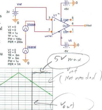
b. Same circuit but now a digital type noise has corrupted the signal. Again plot Vout. Label as is done for report. (4pts)
