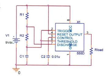
b. (4pt) Using this ratio of R1/R2 and C1 =  $10\mu$ F, calculate the values for R1 and R2 needed to yield a frequency of 20Hz.
