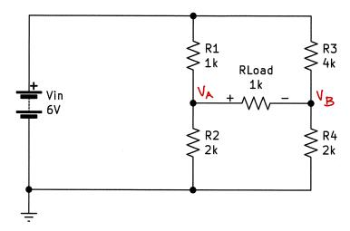
a) Find Thèvenin Voltage for the circuit assuming RLoad as load resistor. {4pts}
