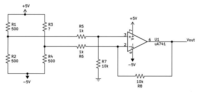
a) If Vout for the Bridge/Amp circuit output is 650 mV, find the value of R3. {8 pts}
