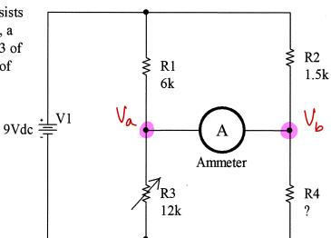
Zero current through ammeter  $\Rightarrow V_a = V_b$
