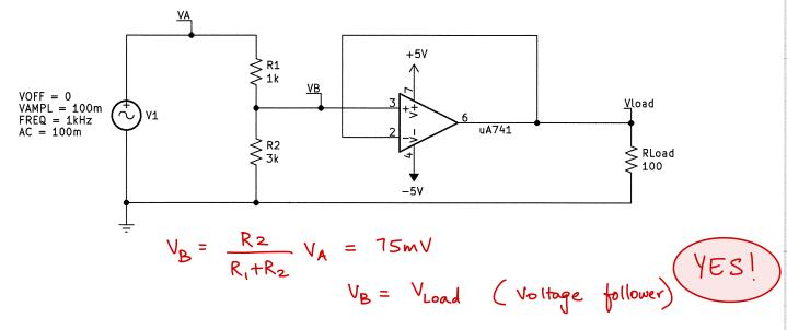
iii. Sketch the voltage waveform, Vload, measured by students X and Y across the load resistor. Also sketch voltage waveforms for VA (same for both students) and pin 3 of op-amp, VB (only for student Y), on the same plot. Label your line plots clearly. Use VloadX, VloadY, VA, and VB for labelling. {4 pts}
