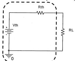
The Thevenin equivalent circuit consists of a voltage source in series with a resistor, which provides a very simple replacement for much more complex circuits. If we have this simple source, analyzing changing loads becomes quite easy.
