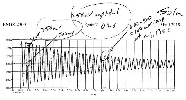
d. The plot shown above represents data taken from the accelerometer on a beam after it has been integrated by an op-amp circuit. Note that there is a dc offset, typical of integration. Find the decay constant α and the angular frequency ω for this data. You must mark the
