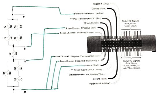
Draw lines between the 2 figures to indicate wires. Both the M2K and the AD2 have the same wiring and colors. W1 is called Signal Generator on the M2K and Waveform Generator on the AD2.
