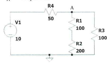
**a.** (6 pts) What is the voltage at point A in the circuit above?
