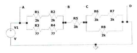
a. (4 pt) It is desired to have the effective resistance of R3 combined with R4 to be 4.8kΩ. Using the table on page 2 of this quiz, standard 5% resistor values, pick resistors for R3 and R4. State the resistance of each. If these resistors have 5% tolerance, what is the 4-band color code for each resistor? You should note that 4.8k isn't a standard value.
