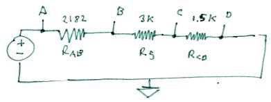
**f.** (2 pts) Using the figure you drew for part e., if V1=4V what is the voltage at point B?
