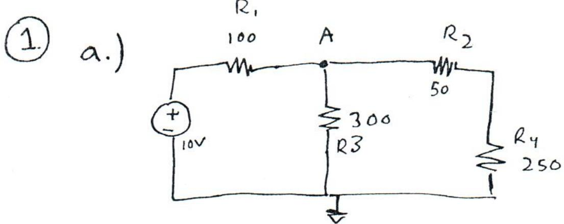
Resistors  $R_2$  and  $R_4$  are in series
