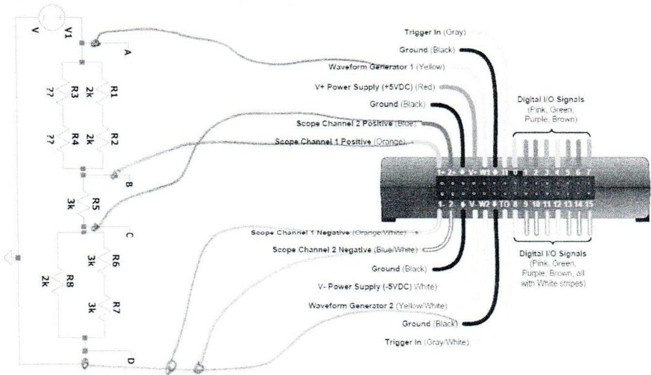
Draw lines between the 2 figures to indicate wires. Both the M2K and the AD2 have the same wiring and colors. W1 is called Signal Generator on the M2K and Waveform Generator on the AD2.
