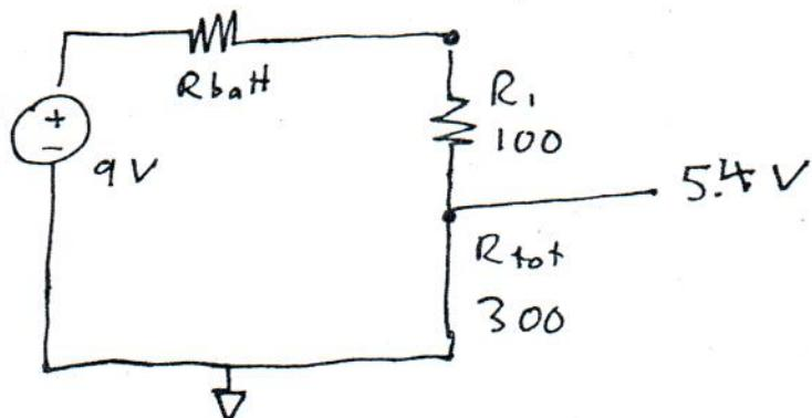
$$V_{\text{out}} = 5.4V = 9V \cdot \frac{300\Omega}{300\Omega + (100\Omega + R_{\text{batt}})}$$
