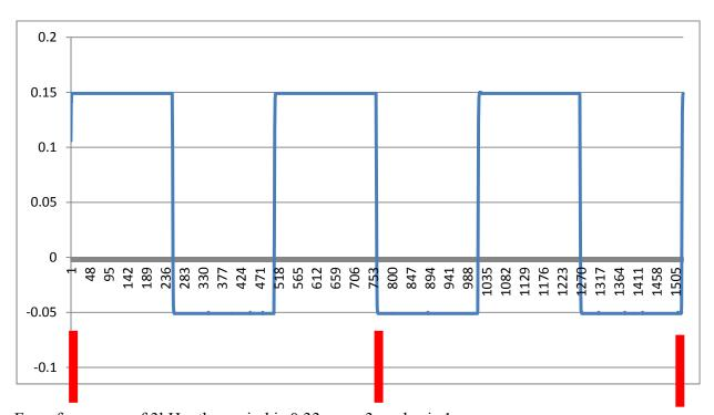
For a frequency of 3kHz, the period is 0.33ms or 3 cycles is 1ms
