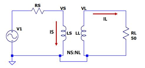
1. (4 pts) With an AC voltage applied to the circuit, you measure VS = 4V and IS = 320mA. If  $Z_{in} = \frac{VS}{IS}$ , what is the value of *a*?
