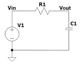
1. (2 pts) V1 is an AC source with varying frequency ( $\omega$ ). Find the transfer function (Vout/Vin) in terms of  $\omega$ , R1 and C1.
