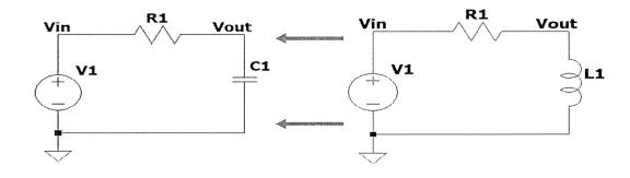
Cascade two filters into one by sharing Vin source & R1
