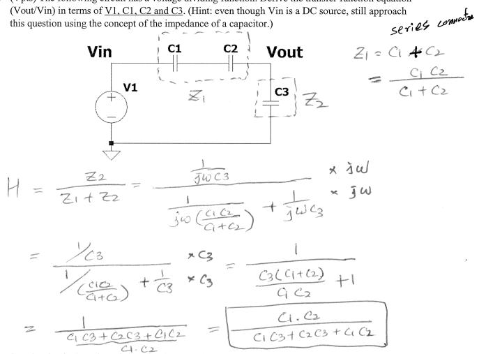
4. (1 pts) What is the value of Vout for the case of V1 = 12V, C1 = 5 $\mu$ F, C2 = 2 $\mu$ F and C3 = 7 $\mu$ F?
