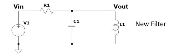
1. (4 pts) V1 input is the same: AC with varying frequency ( $\omega$ ). Find the transfer function (Vout/Vin) of the new filter in terms of  $\omega$ , R1, C1, and L1.
