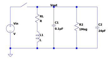
In this case, the value of the input resistance is  $R2 = 1M\Omega$  and the input capacitance is C2 = 24pF. If you needed to find these values specifically for the M2K or the Analog Discovery 2, where would you find them?
