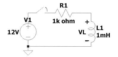
5. (3 pts) What is the current through R1 (1K ohm) before the circuit switches OFF?
