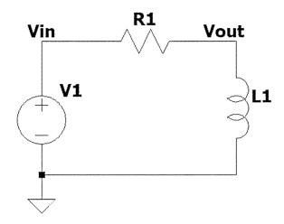
1. (2 pts) V1 input is AC with varying frequency ( $\omega$ ). Find the transfer function (Vout/Vin) in terms of  $\omega$ , R1 and L1.
