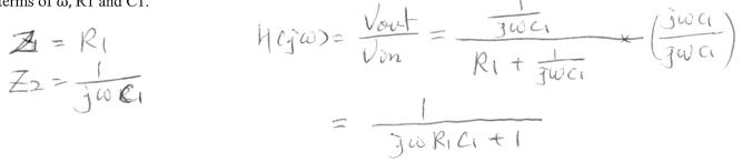
2. (1 pt) What is the simplified transfer function equation at two extreme frequencies (low:  $\omega \rightarrow 0$ , and high:  $\omega \rightarrow \infty$ )?
