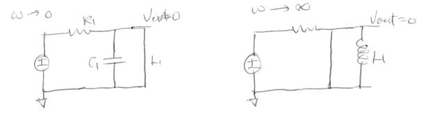
4. (2 pts) Derive the equation for the resonant frequency of this filter. Show your reasoning and assumptions in derivation process. (Hint: at what  $\omega$  does the magnitude of the transfer function have a maximum?  $|H_{max}| = 1$ )
