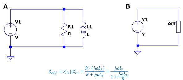
$$\left|Z_{eff}\right| = \sqrt{\left(\frac{j\omega L_1}{1 + \frac{j\omega L_1}{R}}\right) \cdot \left(\frac{-j\omega L_1}{1 - \frac{j\omega L_1}{R}}\right)} = \frac{\omega L_1}{\sqrt{1 + \frac{\omega^2 L_1}{R}}}$$
