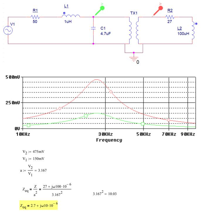
4.6: (4 pts) Draw a 2-component replacement with values for the transformer and attached circuitry (TX1, R2, L2) that will cause the circuit to behave exactly the same in the transformer's ideal region.
