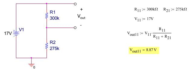
1.2: (4 pts) Reduce the circuit to 3 resistors (in a way to make it easy to find Vout). Redraw the circuit and label the circuit with the appropriate component values. Find the voltage Vout in the circuit below.
