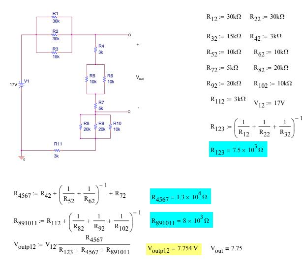
1.3: (4 pts) Using the circuit shown in part 1.2, find the total current from the 17V source (total source current).
